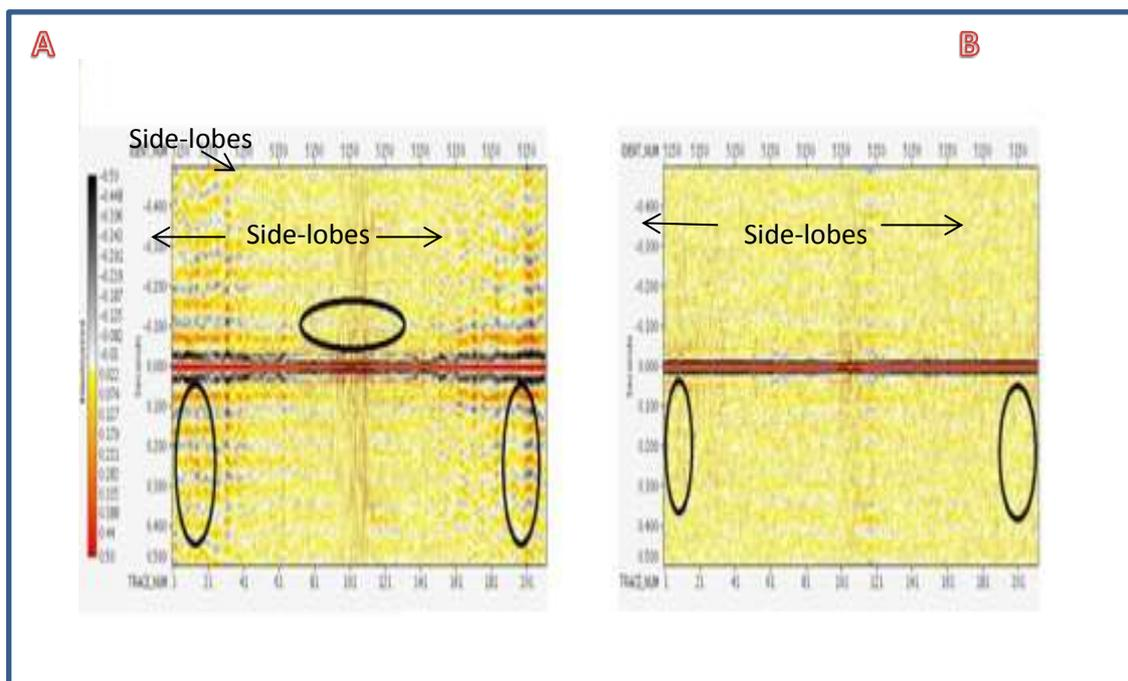
**Figure 4-** illustrates the autocorrelation for line (7Gn 21): (A) Before applying surface-consistent gapped deconvolution, (B) After applying surface-consistent gapped deconvolution
