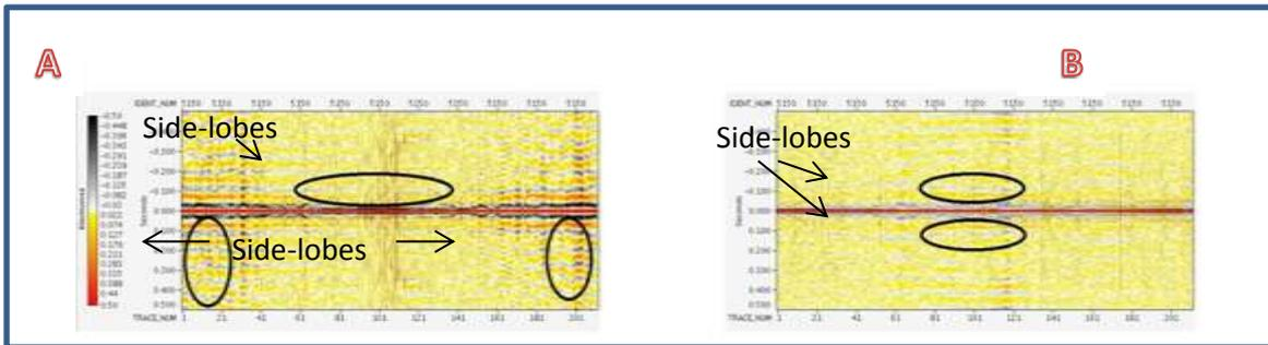
**Figure 7-** illustrate the autocorrelation for line (7Gn 21): (A) Before applying surface-consistent spiking deconvolution, (B) After applying surface-consistent spiking deconvolution
