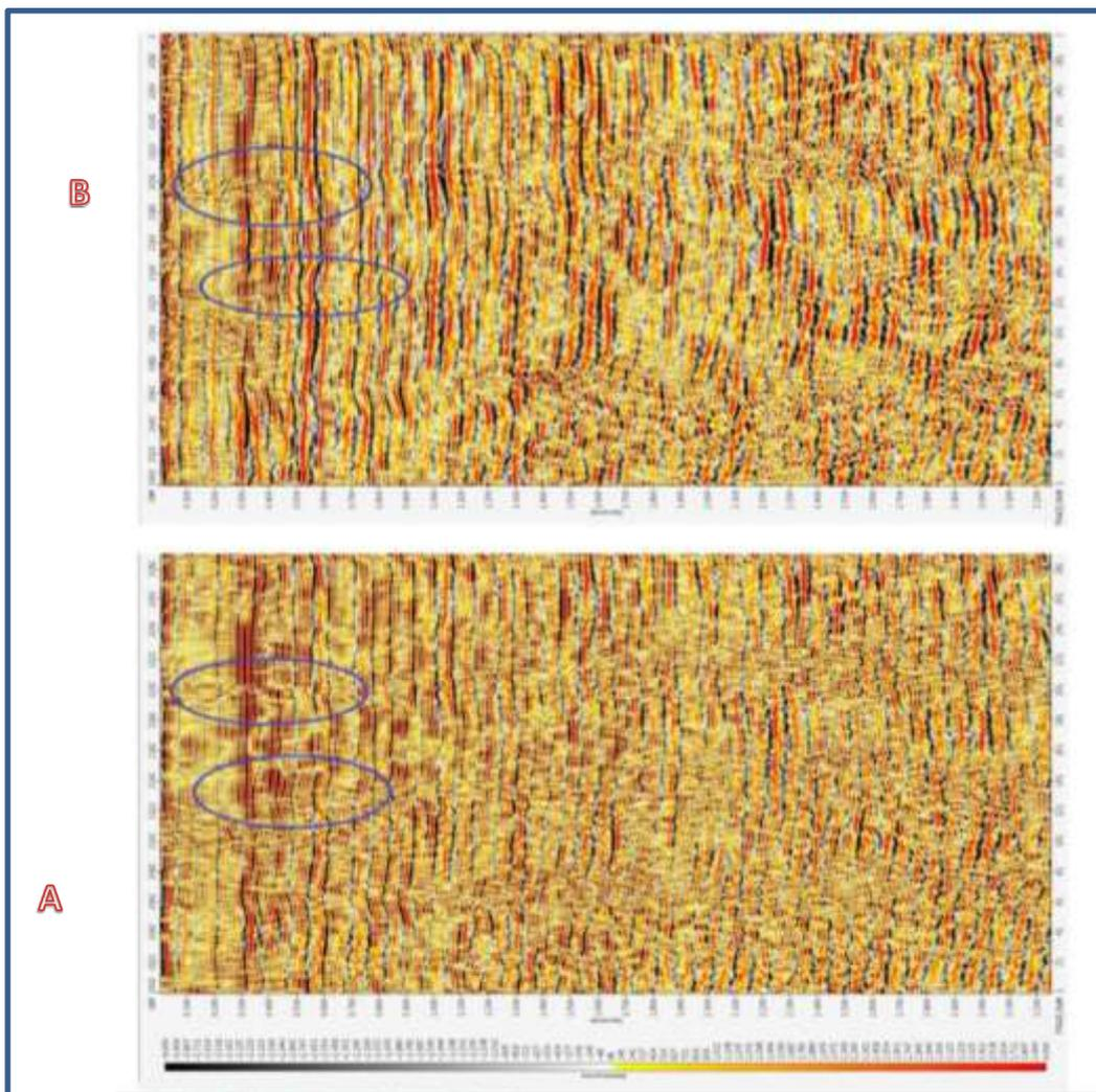
**Figure 8-** Final stacked section for line (7Gn 21): (A) Before applying surface-consistent spiking deconvolution, (B) After applying surface-consistent spiking deconvolution
