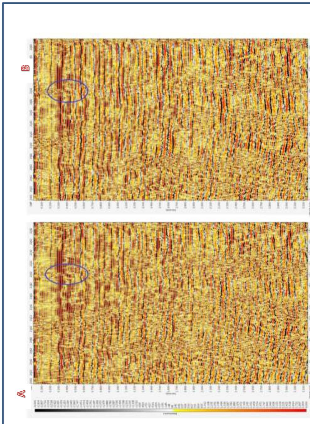
**Figure 5-** Final stacked section for line (7Gn 21): (A) Before applying surface-consistent gapped deconvolution, (B) After applying surface-consistent gapped deconvolution.
