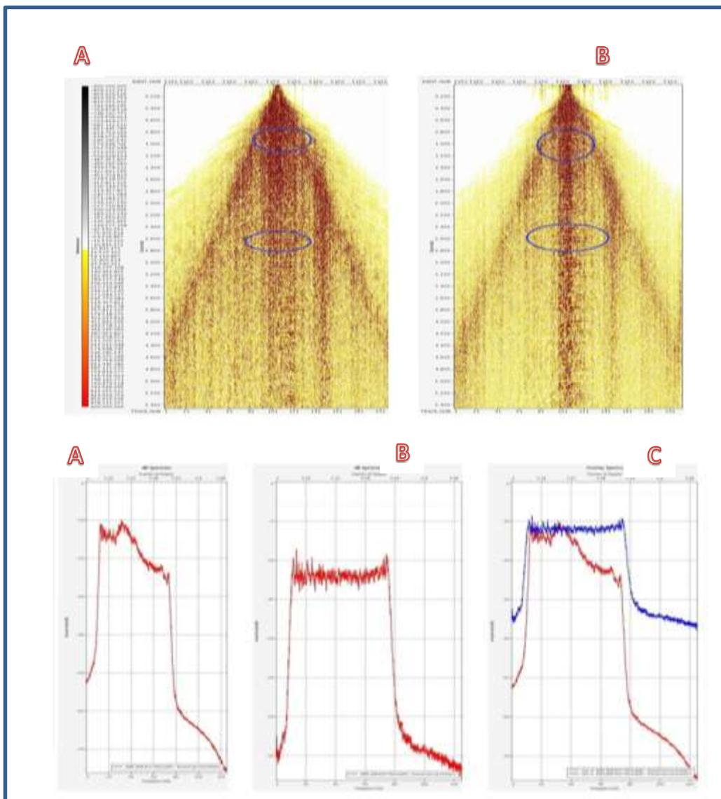
**Figure 6-** shows shots and amplitude spectrum for line (7Gn 21): (A) shot and spectral analysis before applying surface-consistent spiking deconvolution, (B) shot and spectral analysis after applying surface-consistent spiking deconvolution, (C) overlay spectral analysis, the red line before deconvolution and the blue line after applying deconvolution.
