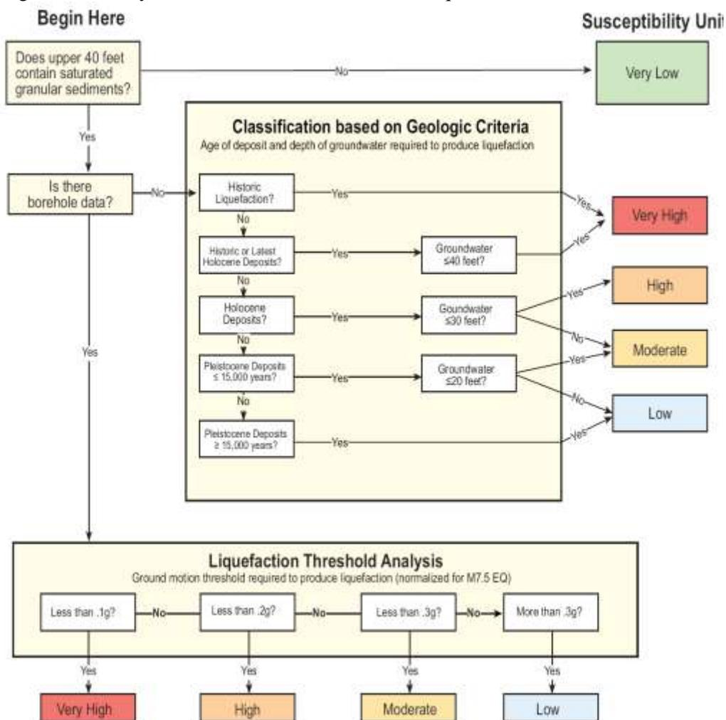
**Figure 3-** Flowchart to determine the risk of liquefaction in the coastal areas.
